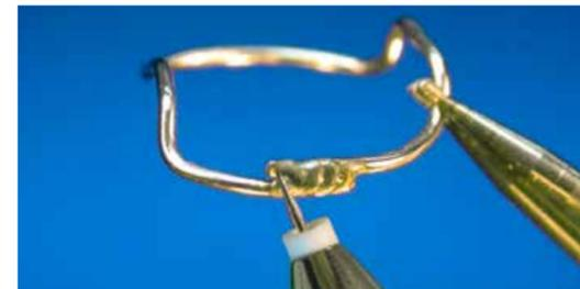
Connecting stainless steel wires
